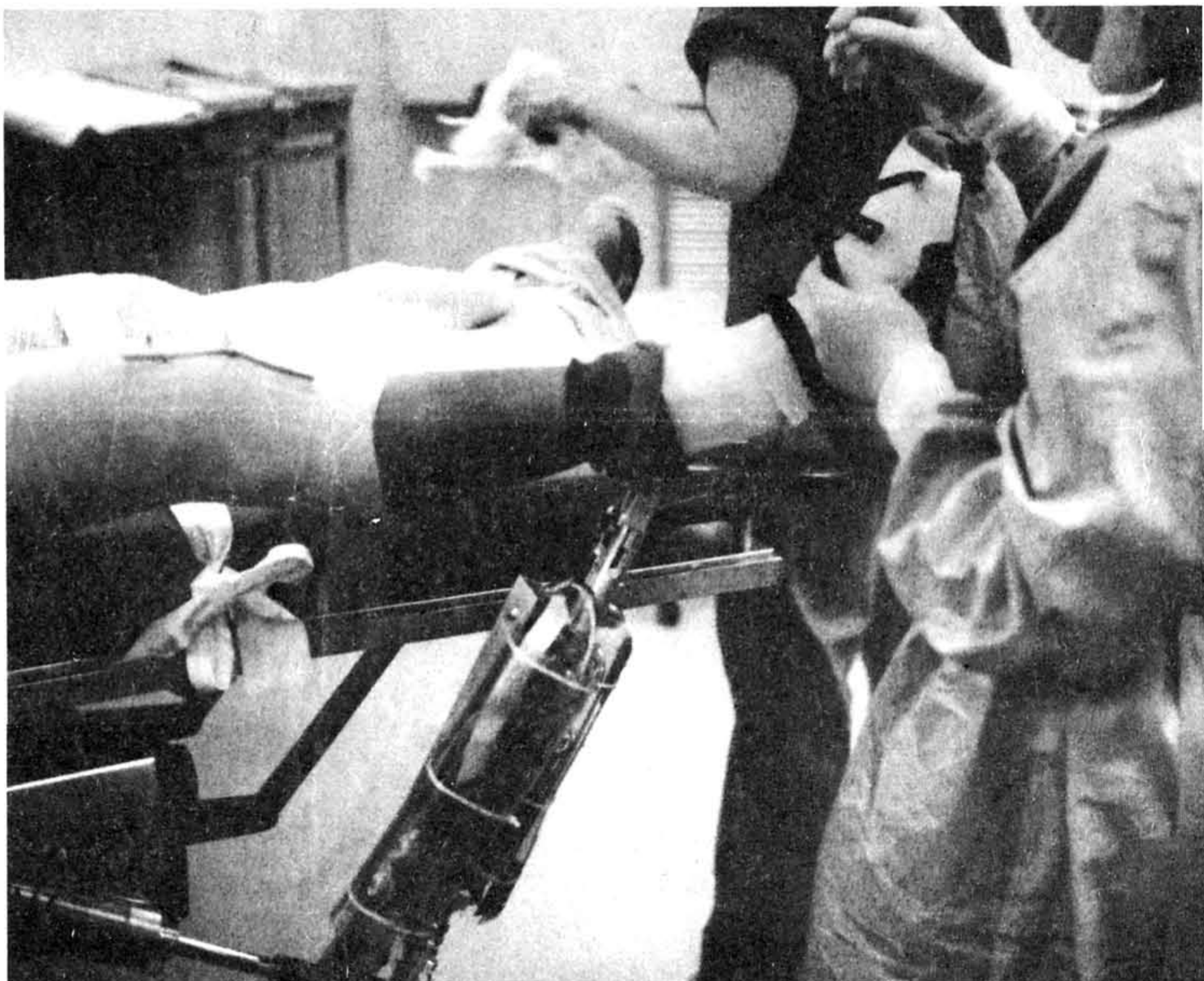
THE ARTHROBOT, an advanced robotic assistant for orthopedic surgery, manipulates and positions the patient's leg on voice command.
